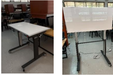
Figure 10: Sitting and Standing Screening Mode of the Build and Tested Adjustable Desk
