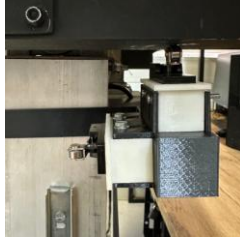
Figure 14: 3D Printed Limit Switch Bracket
