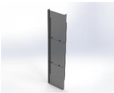
Figure 3: Telescopic Leg Housing
