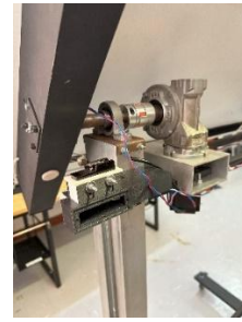
Figure 12: Worm Gearbox and Stepper Motor Assembly
